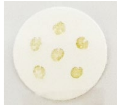
Fig. 5 Solid-state sample image of S. armatus cells with optimal conditions as the volume of sample 5 \mu\text{L} fabricated onto GF/C™ filter and dried at room temperature for 30 min
